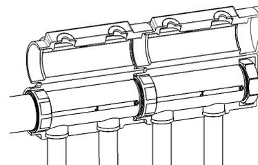
To install the shells with the supports, art. 7480-7550, use the cutting guide in the shell that corresponds to the supports, as shown in the picture.
