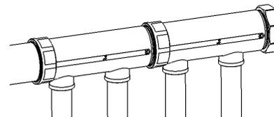
2. To connect insulated manifolds, simply cut the shell at the marked lines already drawn inside the shell.
