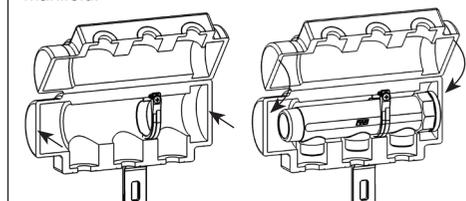
3. Close the shell so as to seal the inner surface to the manifold. Fix the shell by means of adhesives already placed on the shell
